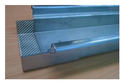
4. Reset the channel section back in place on the sealant (ensure the joining channels meet) and remove any excess sealant that seeps through the joint into the channel.
